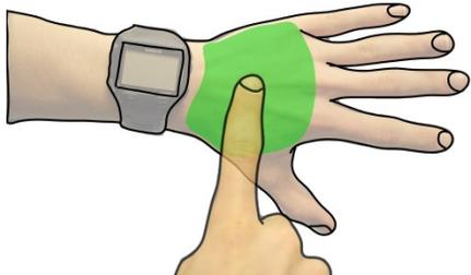
**Figure 2.** By moving the interaction to the side of the device, the interaction area can increase significantly and remove the problem of occlusion. The green area now indicates a much larger interaction space.
