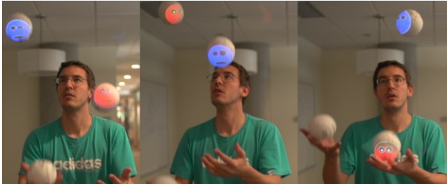
Figure 1. The Juggling Display; projection alignment on fast-moving objects through software-based latency reduction.
